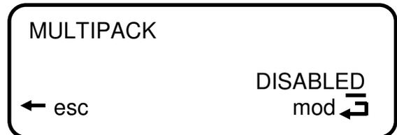
**NOTE:** Enabling the multipack feature allows specific product size data to be entered into the PLC. This may be necessary when unusual package shapes do not register properly in the photoelectric cells.
