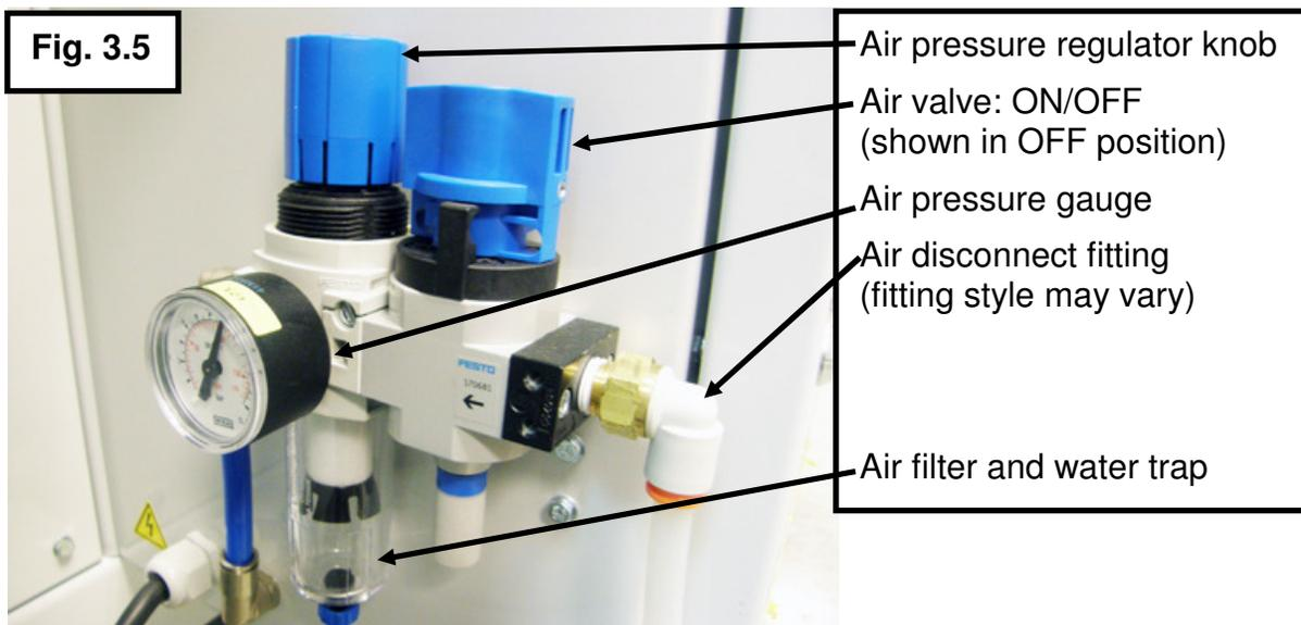
**NOTE:** Air fitting base is CLAMCO part number 390-000074. The elbow fitting is part number 785-64
