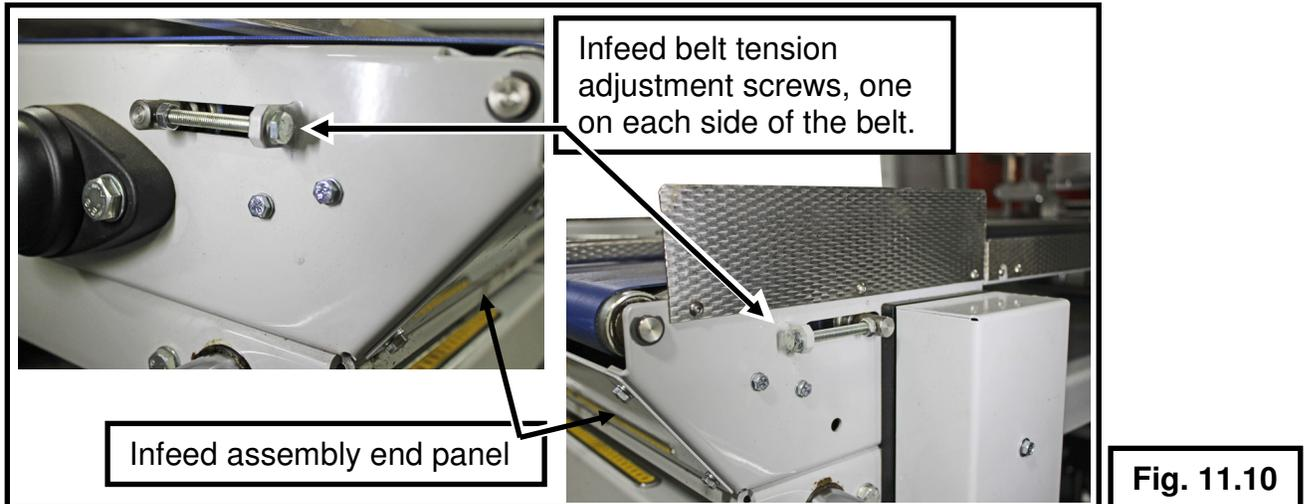
4. Loosen the jam nuts and turn the adjuster screw to relieve as much tension from the belt as possible.
