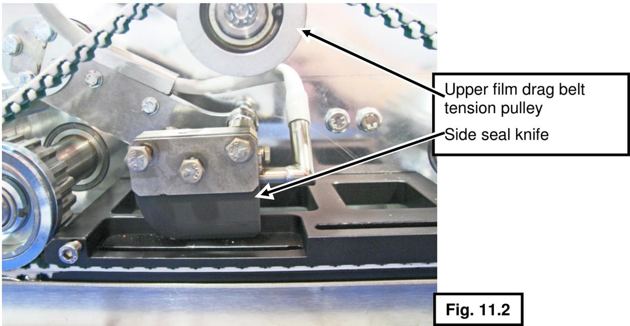
6. Remove the upper film drag belt tension pulley using a 13mm wrench. A crescent wrench may be needed for the hex shaft.
