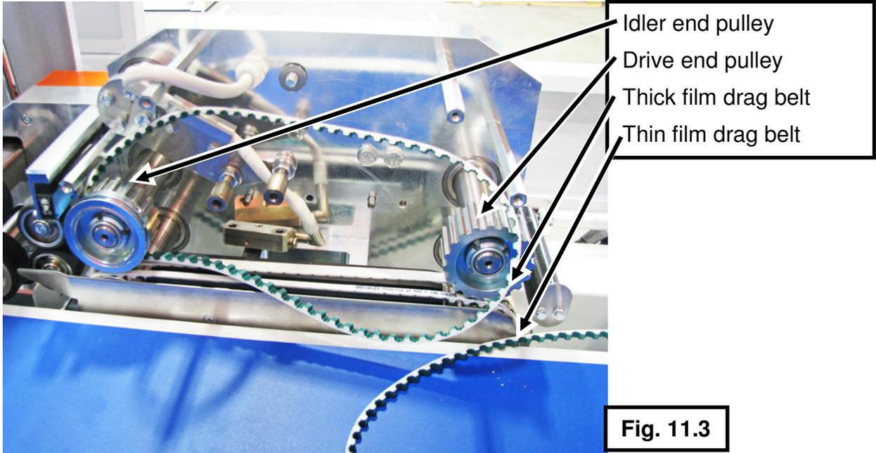
8. The wide upper film drag belt will be trapped on the idler pulley by a collar. Remove the collar using a 2mm hex key. See Fig. 11.4.
