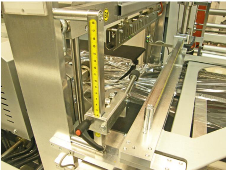
Raising film guides can be used to help open the pocket of film that the product is pushed into by the infeed conveyor.
