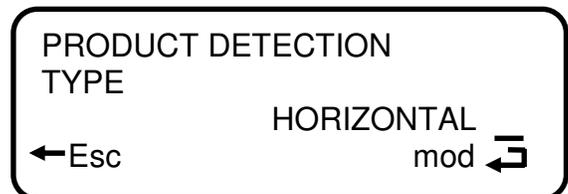
5. Horizontal- Use the horizontal photo cells to detect packages that are more than 2cm (3/4") tall.
