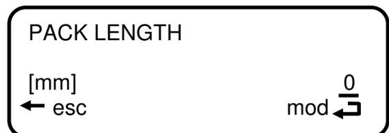
**NOTE:** If a package length is specified in this field, but the Multipack feature is disabled, the length entry will be used as a maximum limit for the photoelectric package detection. If a package is detected that exceeds this length, an "ANOMOLOUS PACK" error will be displayed on the screen.
