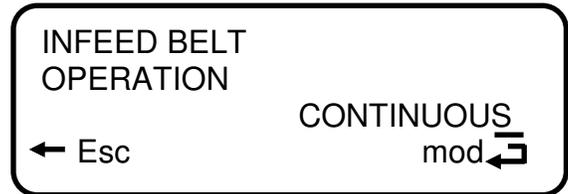
5. Continuous- The infeed belt runs until the product detection photo cells sense that the product has passed the seal jaws.
