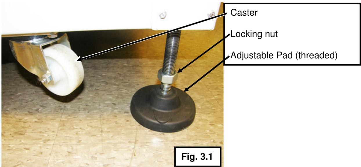
**NOTE:** When used with a heat tunnel, the 6800CS should be adjusted so that the end of the takeaway conveyor is 1mm lower than the tunnel conveyor.
