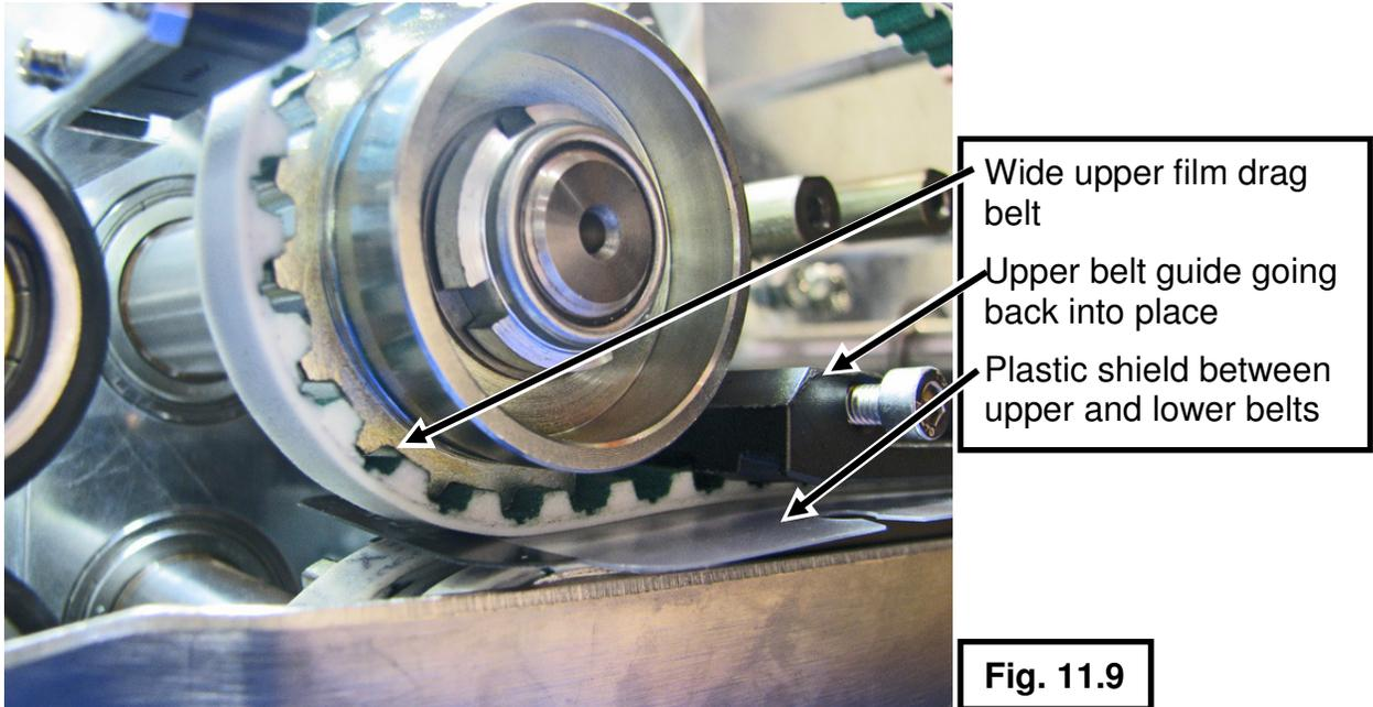
21. Once the upper belt guide is started over the dowel pins, start and tighten the socket head caps screws to draw it into place. As the groove for the thin film drag belt moves in, start the thin film drag belt through the groove and around the pulleys and collar.
