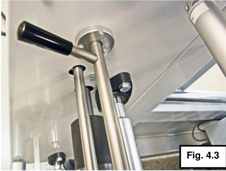
4.1.10 Move the perforation wheels out of the way. Turn the lock levers counter-clockwise to loosen them, and clockwise to lock them in place.
