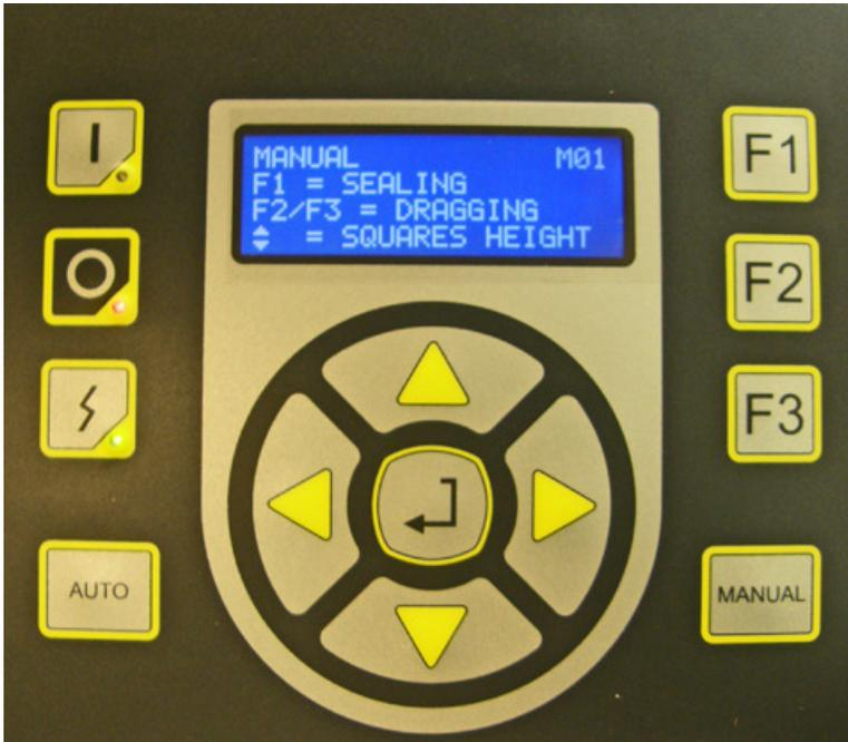
7.1.2 **Energize Button:** With power connected and the main switch ON, the Energize button turn the sealer on.
