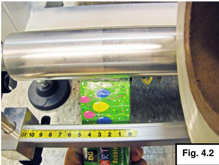
**NOTE:** The square bar that supports the film guides is marked in centimeters. Zero on the measuring scale is even with the tip of the inverting plows.
