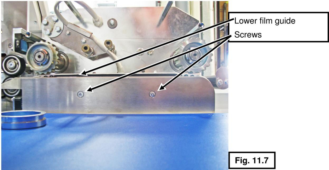
14. Cap screws fasten the hexagonal mounting posts for the lower film guide to the side sealer frame. Remove the cap screws holding the two lower hexagonal mounting posts to the side seal frame using a 7mm socket.
