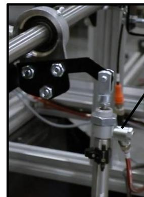
Flow control valve controlling the actuator extend speed
