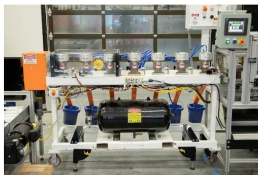
Figure 1: Hole Punch Assembly
