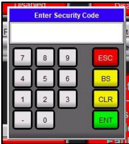
The operator should use the numeric portion to enter the proper 4-digit security code for the appropriate level of clearance. The code for the MAINT group is 1900. Once the correct code has been entered, the MAINTENANCE screen will be displayed:
