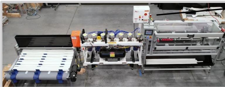
The Stack Light can be seen here – just above the HMI Display
