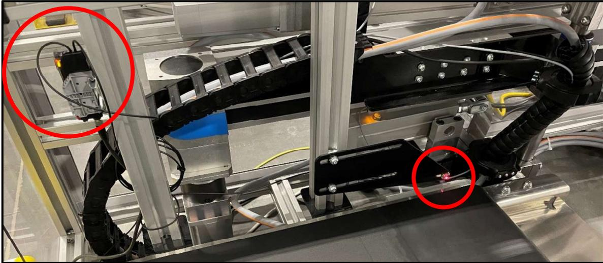
*Figure 22. Keyence fiberoptic thru-beam sensor detects bags along conveyors, providing signals to properly control the flow of bags in the system.*
