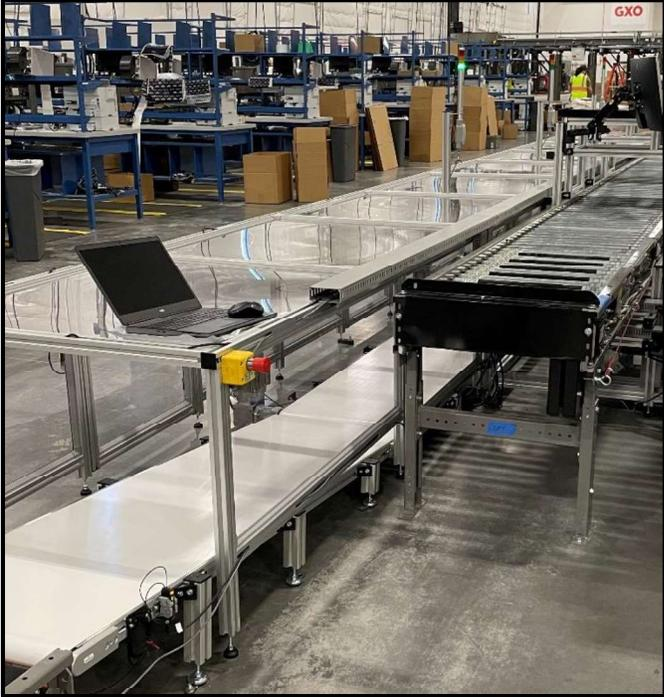
Figure 3. Outbound E-stop on main enclosure.
