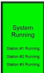
The HOME SCREEN DISPLAY icon will display this indication when the system is running. It will also indicate which stations are running.
