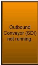
If the outbound conveyor stops, this message will be displayed when a bag reaches the discharge part of the transition conveyors.
