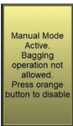
This message will display if the system is switched to "Manual Mode". An orange button will display to switch the system back to Auto Mode and process bags.
