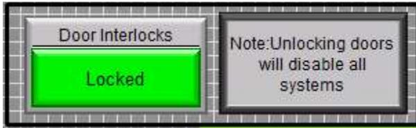
The “Door Interlocks” button toggles between “Locked” and “Unlocked”. By unlocking the door interlock, you will gain access to the conveyor transition system. Make sure to close all doors firmly after opening any door. The interlocks status lights will also indicate its status as follows.
