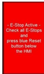
Should an E-Stop be pressed anywhere on the system, the HOME SCREEN DISPLAY icon will be displaying the message shown to the left.
