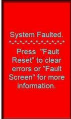
If any system faults are active, they should be cleared by pressing the FAULT RESET button. Additionally, all of the access doors into transition conveyor area (if they are indicating an UNLOCKED state) should be locked by pressing the DOOR INTERLOCKS icon. This may require proper positioning of the door locks prior to attempting to lock the doors.
