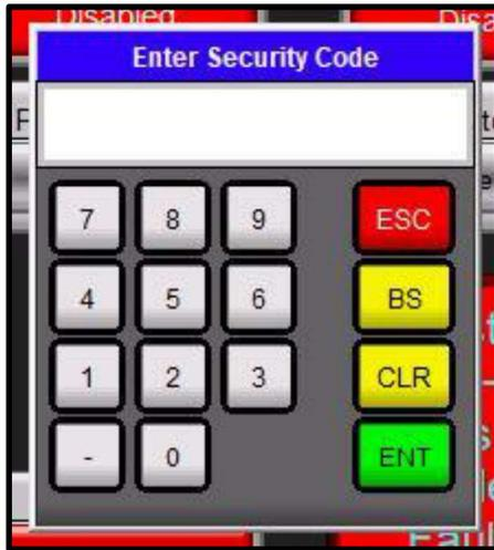
The operator should use the numeric portion to enter the proper 4-digit security code for the appropriate level of clearance. The code for the MAINT group is 2222. Please note that the only difference between MAINT group and ADMIN group is that the ADMIN group can read and edit fault history, while MAINT group can read (but not edit) fault history. Once the correct code has been entered, the desired screen will be displayed.
