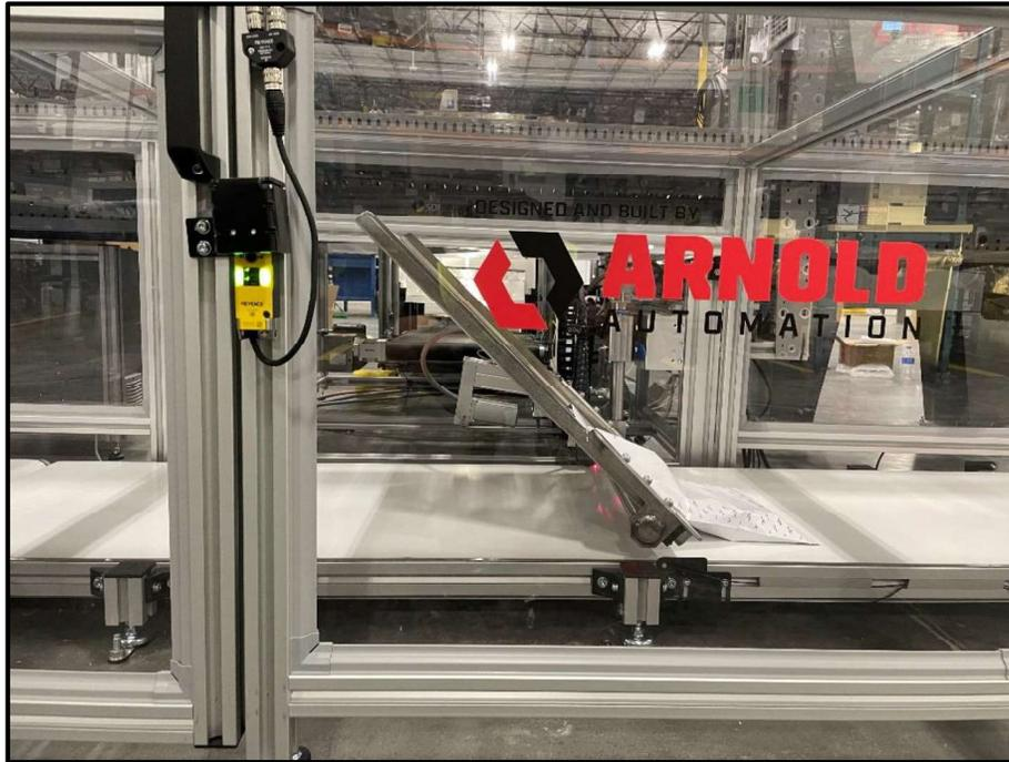
*Figure 24. Keyence door locking switch lit solid GREEN indicating that the door is locked.*
