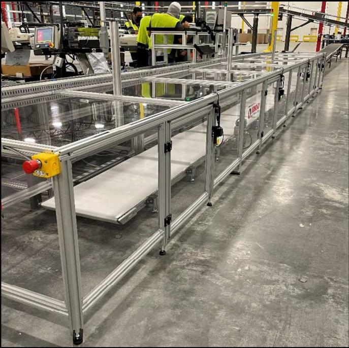
Figure 4. Inbound E-stop on main enclosure.
