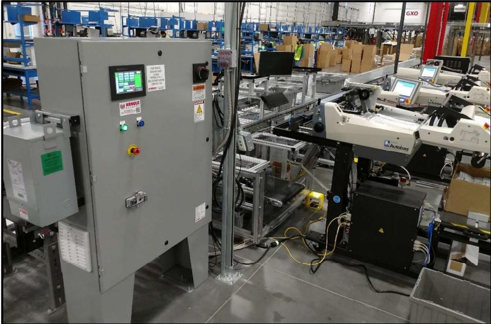
Figure 2. E-stop (red and yellow button) on main electrical enclosure.
