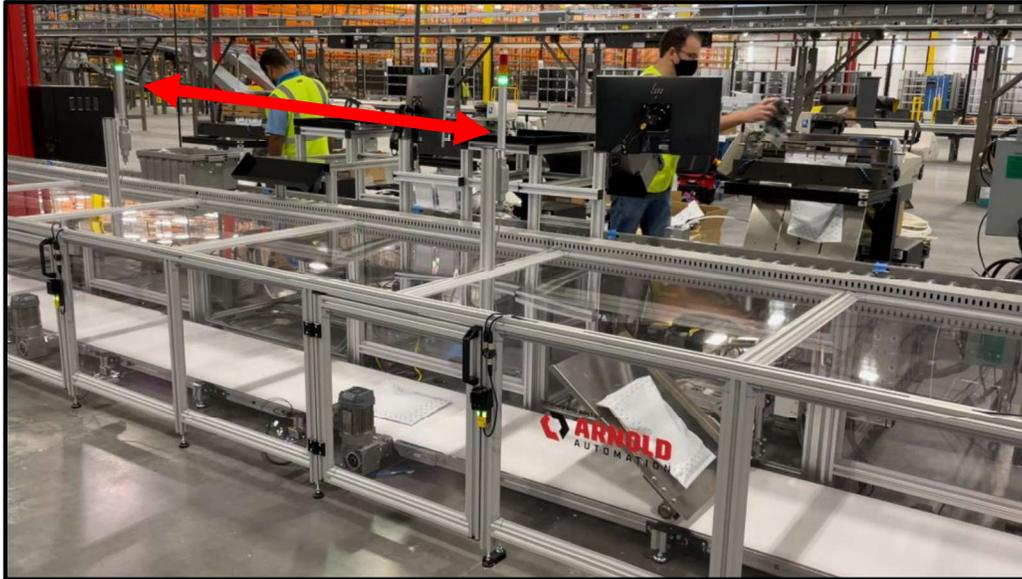
Figure 7. Tower lights lit GREEN during normal operation.
