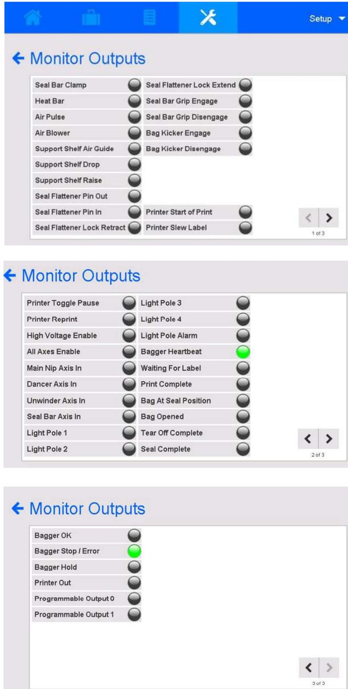
FIGURE 4-17. D DIAGNOSTIC OUTPUTS, PAGES 1-3
