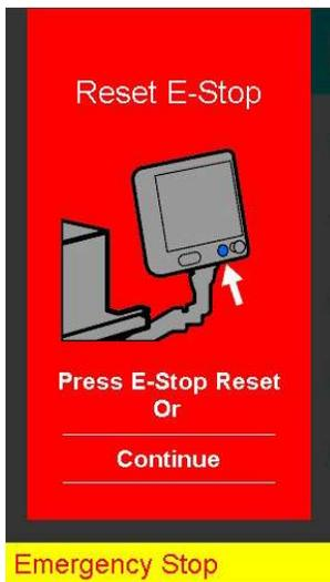
FIGURE 3-4. RESET E-STOP DISPLAY
