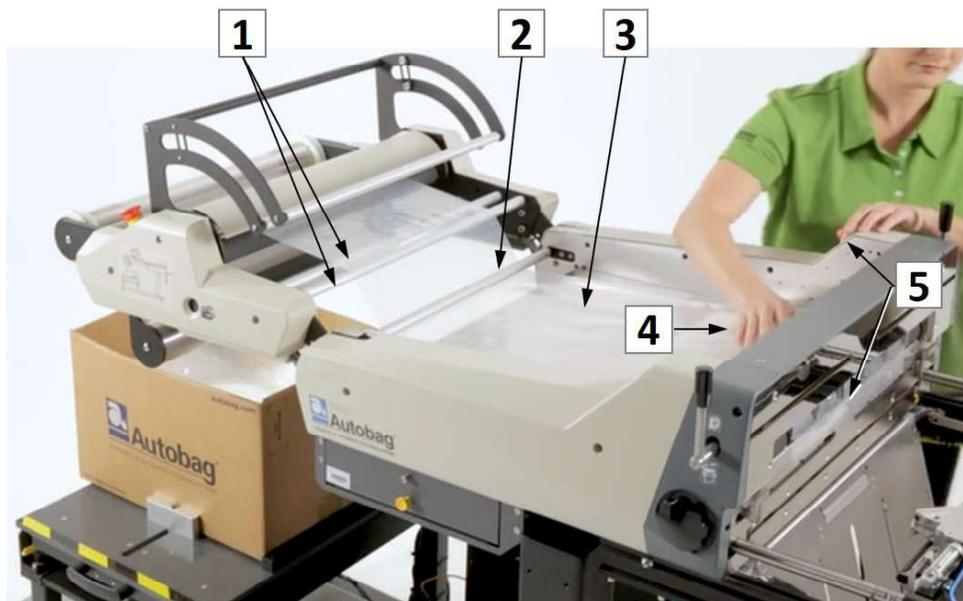
FIGURE 3-21. BAG WEB THREADING DETAIL
