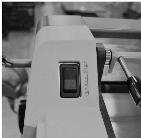
*FIGURE 3-19. AUTOTHREAD SWITCH*
