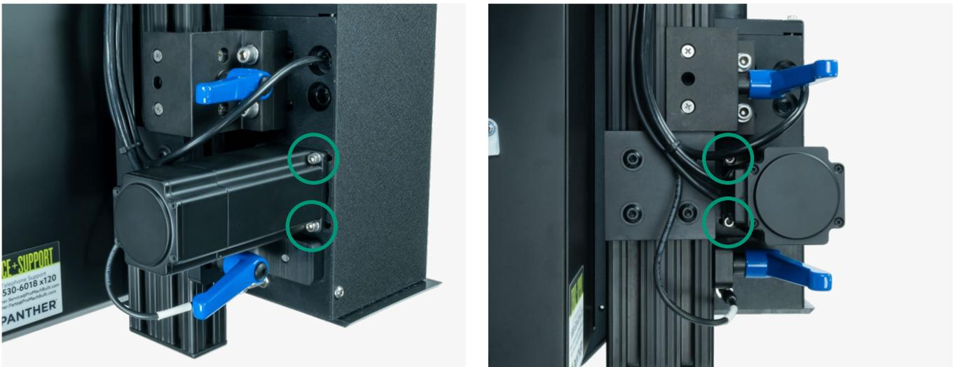
8. Move the applicator rack up and down to ensure the motion is smooth and does not stall in any location. Check the applicator rack for any broken or damaged teeth. Clean any debris or build up within the teeth.
