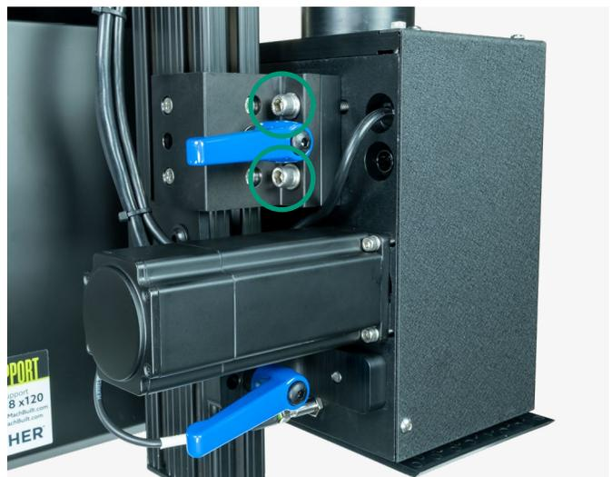
12. Loosen the vertical adjustment lock handles, located on the back of the Predator main plate.
