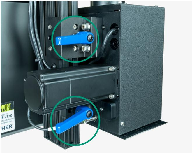
13. Adjust the vertical position of the tamp head so that the print engine peel bar splits the bevel on the tamp head. **Note: This will require adjusting the fixed mounting bolt that the slide assembly rests on. You should position the surface of the tamp head approximately 1/16" below the position where the labels feed out.**
