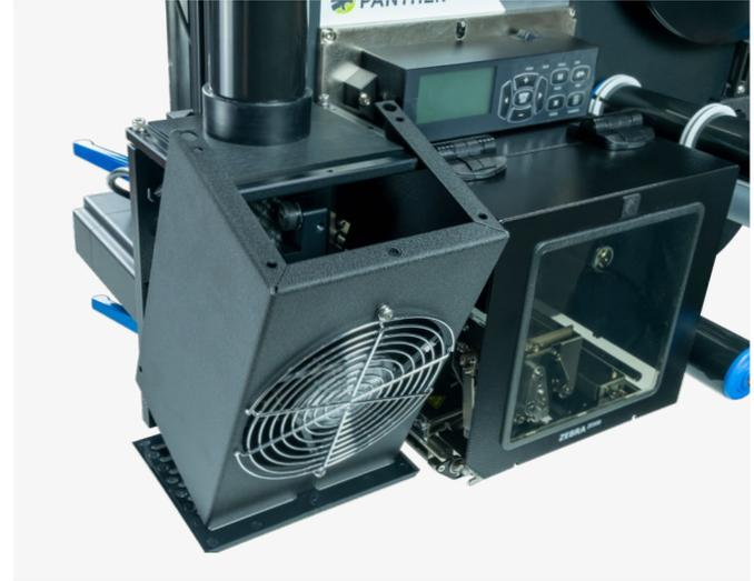
2. Remove fan shroud and disconnect the power wires from the fan.
