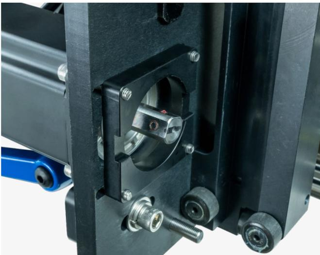
6. Using even pressure on the motor, push the applicator drive motor back towards the applicator rack.
