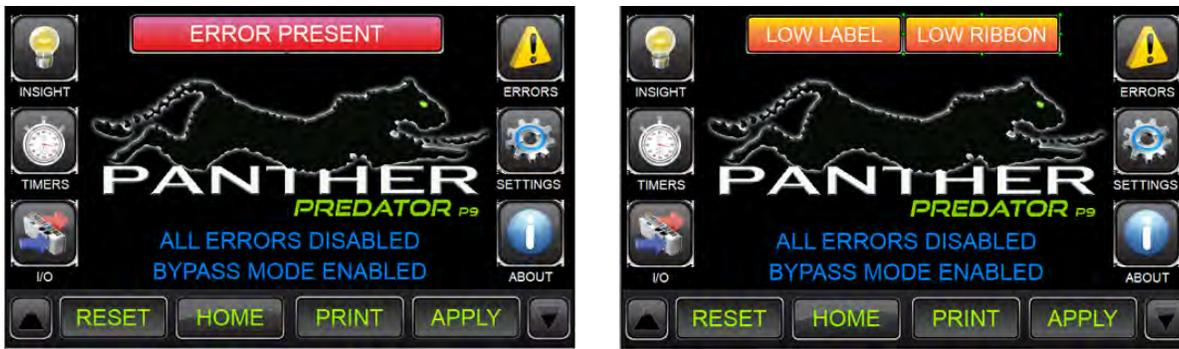
1. If the labels are low or the ribbon (if used) is low, the respective lamp within the status indicator bar on the home screen will illuminate.
