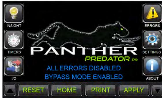
The Panther Predator is provided with six STANDARD operator and maintenance screens. (Additional or customized data may be displayed at the customer's request.) These screens are all accessible from the Panther Home Screen. The settings screen allows for the option to view the settings as icons or in list fashion.
