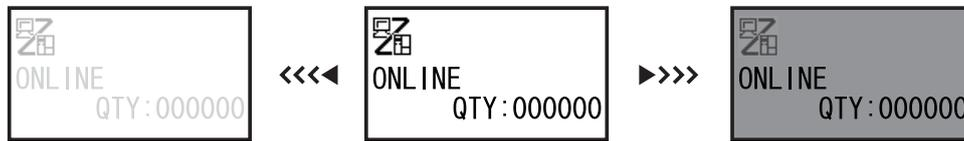
You can adjust the brightness in thirty-two steps (sixteen left and sixteen right). The brightness changes one step for every press of the ◀ button or ▶ button.
