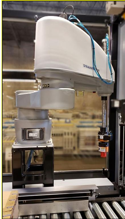
**Figure 26 - CASi-IBOD Box Cutter Robot**
