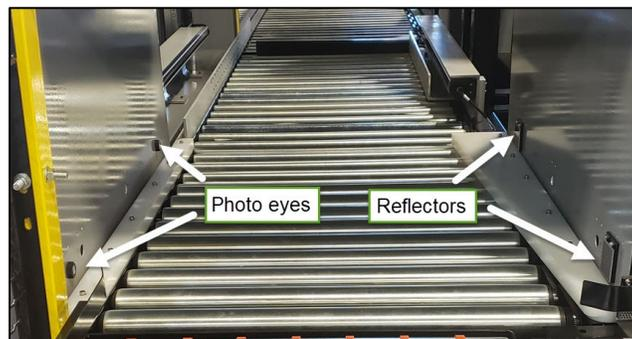
**Figure 21 - CASi-IBOD - Infeed Photo Eyes and Reflectors**
