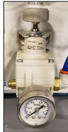
**Figure 143 - Precision Regulator (for collision sensor)**
