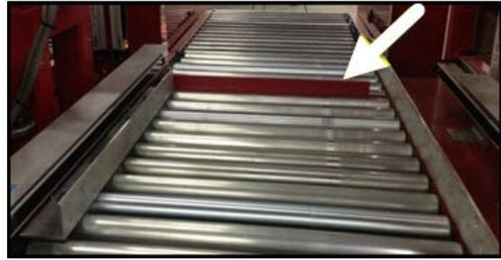
**Figure 32 - Blade Stop Deployed**
