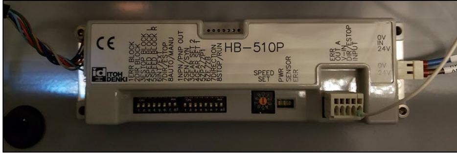
Figure 22 - CASI-IBOD - Motor Drive Card
