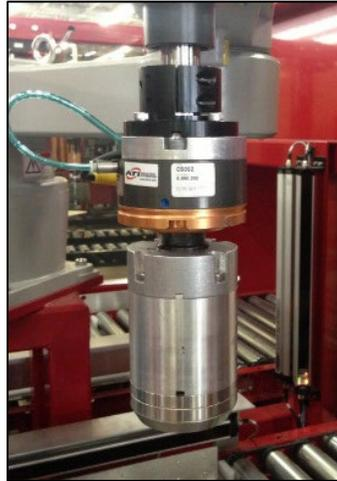
**Figure 147 – CASi-IBOD Box Cutter Robot Collision Tool/Test**
