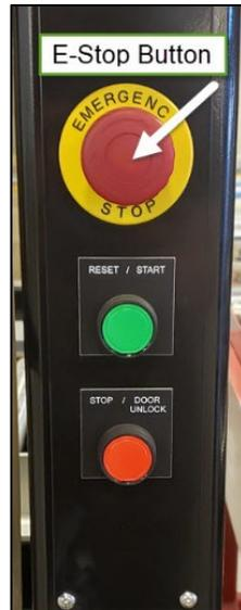
Figure 53 - IBOD Frame E-Stop
