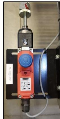
**Figure 51 - Close-up E-Stop Rope Pull Reset Button**
