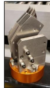
**Figure 146 - Tape Cut Tool**
