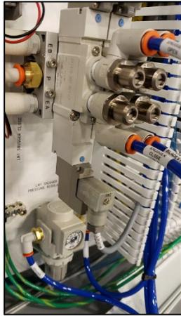
**Figure 140 - Component Solenoid Valves**
