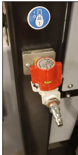
**Figure 59 - IBOD Main Air Shutoff**
