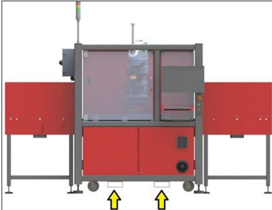
**Figure 41 - CASi-IBOD Forklift Slots**
