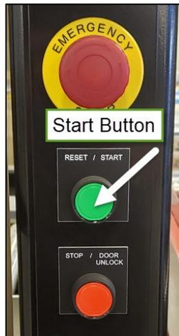
Figure 47 - IBOD Frame Control Start
