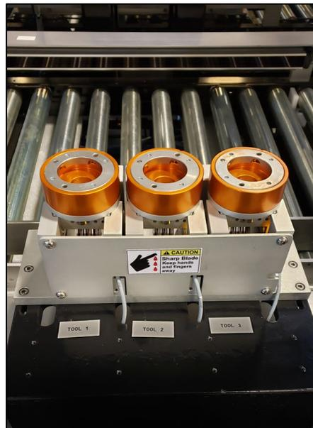
**Figure 27 - CASi-IBOD Robot Tool Changer rack, shown with 3 extra tape-cut tools**
