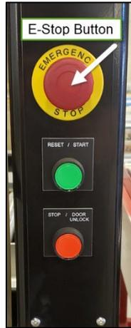
**Figure 48 - IBOD E-Stop Frame Button**
