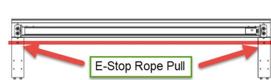
**Figure 2 – Conveyor Rope Pull locations (Optional)**
