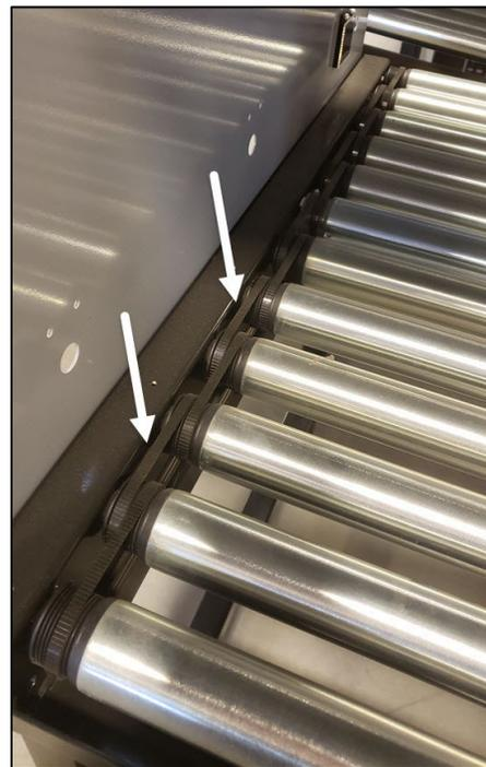
Figure 24 - CASI-IBOD Infeed Roller Belts
