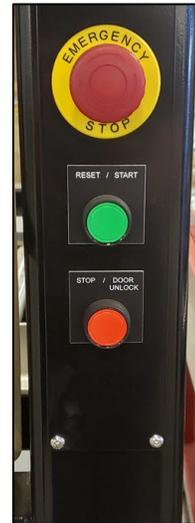
**Figure 36 - Frame Control Buttons**
