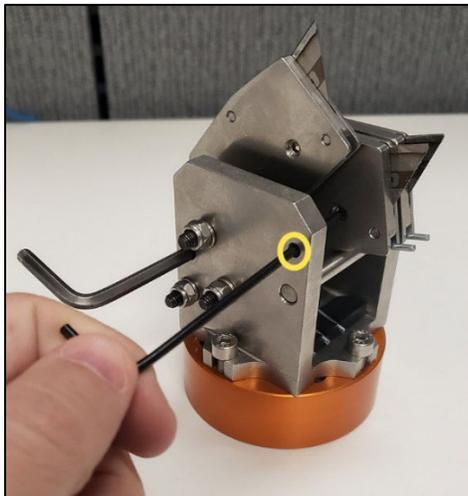
Figure 53 - Remove the Second Blade
