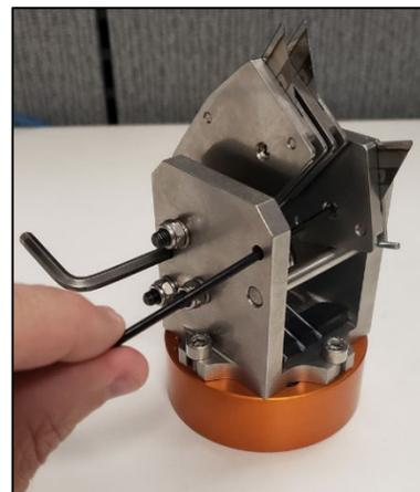
**Figure 57 - Pin Third Blade Holder Down**
