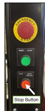
**Figure 106 - Mechanical Stop Button**
