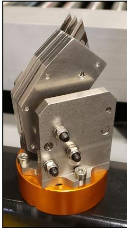
**Figure 45 - Tape Cut Tool Head**
