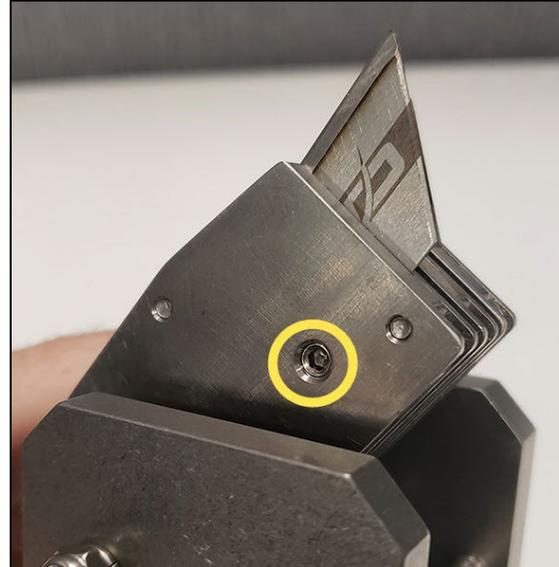
Figure 65 - Correct Set Screw Depth
