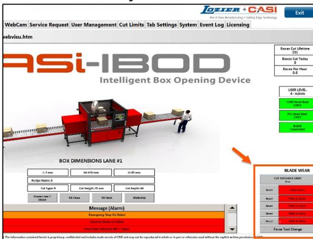
Figure 100 - Blade Wear Section
